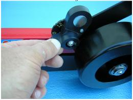
Your rollers are fitted with a magnetic resistance unit which may be set to 4 different positions. Rotate the arm as shown to the numbered stops. The zero number is "off" and the resistance goes higher for the each of the settings 1 thru 3
